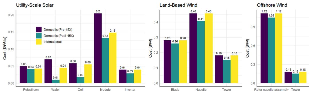
**Figure 1. Estimated production costs for solar and wind components that are globally- and domestically-produced. Costs for domestically-produced components are reported prior to and after receiving the 45X tax credit. Production costs may differ from final product pricing. Refer to SI Table S17 for details.**
