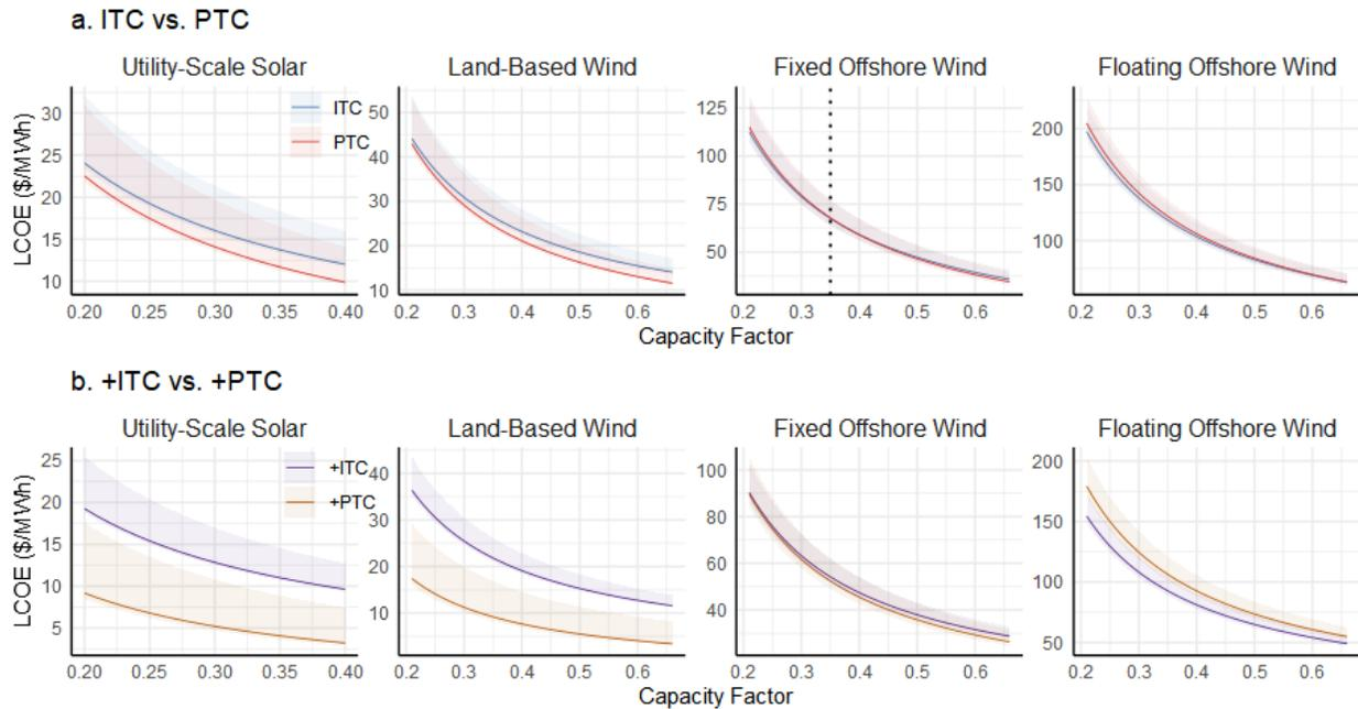
**Figure 3. Levelized cost of electricity (LCOE) for each technology with respect to capacity factor. The impact of capacity factors is evaluated for the *base* (a) and *bonus* (b) tax credit rates. The LCOE for 2030 is depicted by solid lines, while the shaded regions represent the potential range of LCOE values from 2023 to 2050. The vertical dotted lines represent capacity factors, where the minimum LCOE shift occurs between policy scenarios.**
